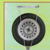
**PORTE ROUE DE SECOURS SOUS CHÂSSIS**
